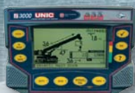
Safe load indicator
