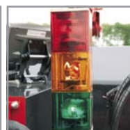
Overload warning lamps + auto stop + alarm
