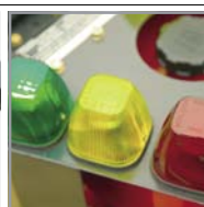
Overload warning lamps + auto stop + alarm
