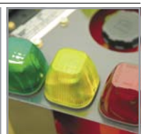
Overload warning lamps + auto stop + alarm
